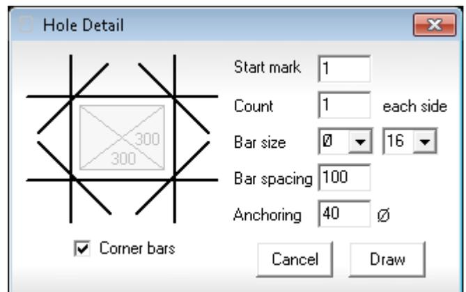
A settings dialog appears on screen. Anchorage should be measured outside the hole edge.
